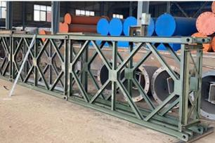
The bridge body components can be loaded into small trucks. A convoy of several trucks can move everything needed for a complete bridge. No special tools, skills or heavy equipment are required.
