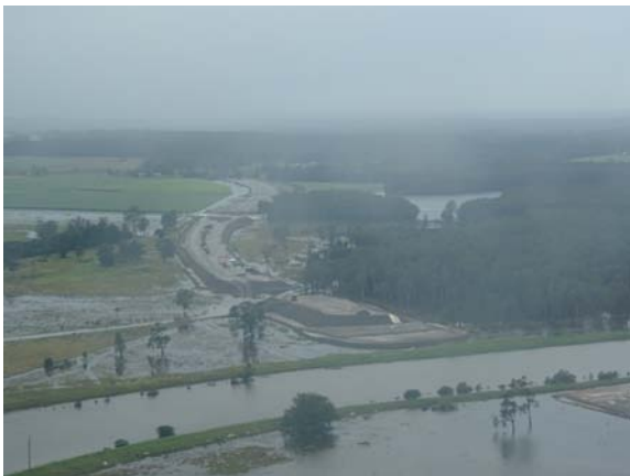
Fig 8. Water banked on the western side of the carriage way embankment, north and south of the Canal, after heavy rain in 2017
