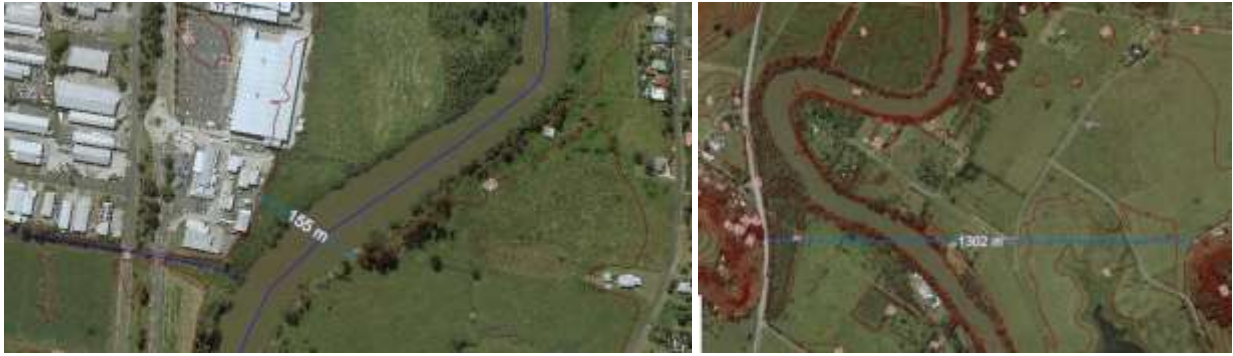
Figure 15. Stream widths at the 10m contour for two choke points below Lismore, (left) 155m just south of the Masters/Spotlight roundabout, and (right) 1300m at Sandy Point with numerous obstructions.
