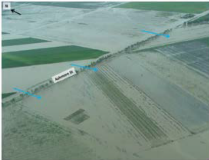
Figure 32. Flows overtopping Ashmore Street in the 2010/11 floods (Water Technology , 2014)
