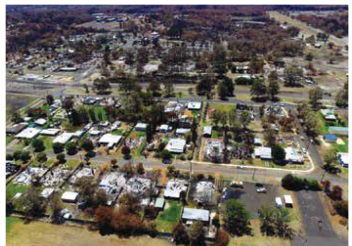
Below: Green lawns around destroyed houses can prevent fire spread (source: ABC News)
