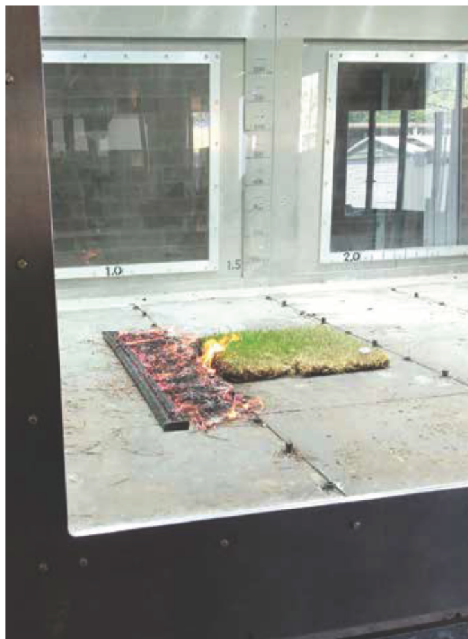
Living turf not sustaining ignition
