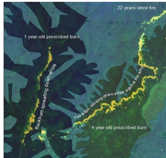
Figure 5 | Western edge of the Green Wattle fire spreading down-slope through a 4-year-old prescribed burn. A 1-year-old prescribed burn lies in its path, but no confidence has been placed in this, and a backburn has been lit from the trail at its centre. The backburn is spreading down-slope through the 1-year-old fuels, with no difference in depth of the flaming edge compared to the 22-year-old fuels at the top of the image.
