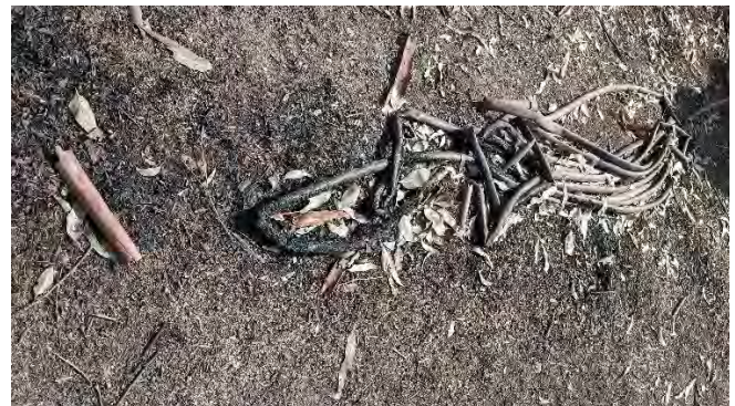
Fire hose on dam pump - burnt
