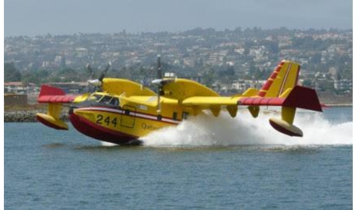
Figure Six: Canadair CL415 “Super Scooper”. Note ability to drop at low altitude.
